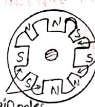
inter practice. In this method reversing e.m.f required to neutralize Reactance voltage is induced in the coil undergoing commutation by using small poles fixed to the yoke and placed in between the main poles. i.e along geometrical neutral axis. These poles are called Interpoles. practically interpoles are placed in b/w the main poles.
